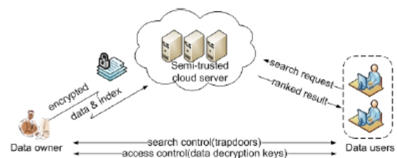
Fig. 1: Architecture of the search over encrypted cloud data
